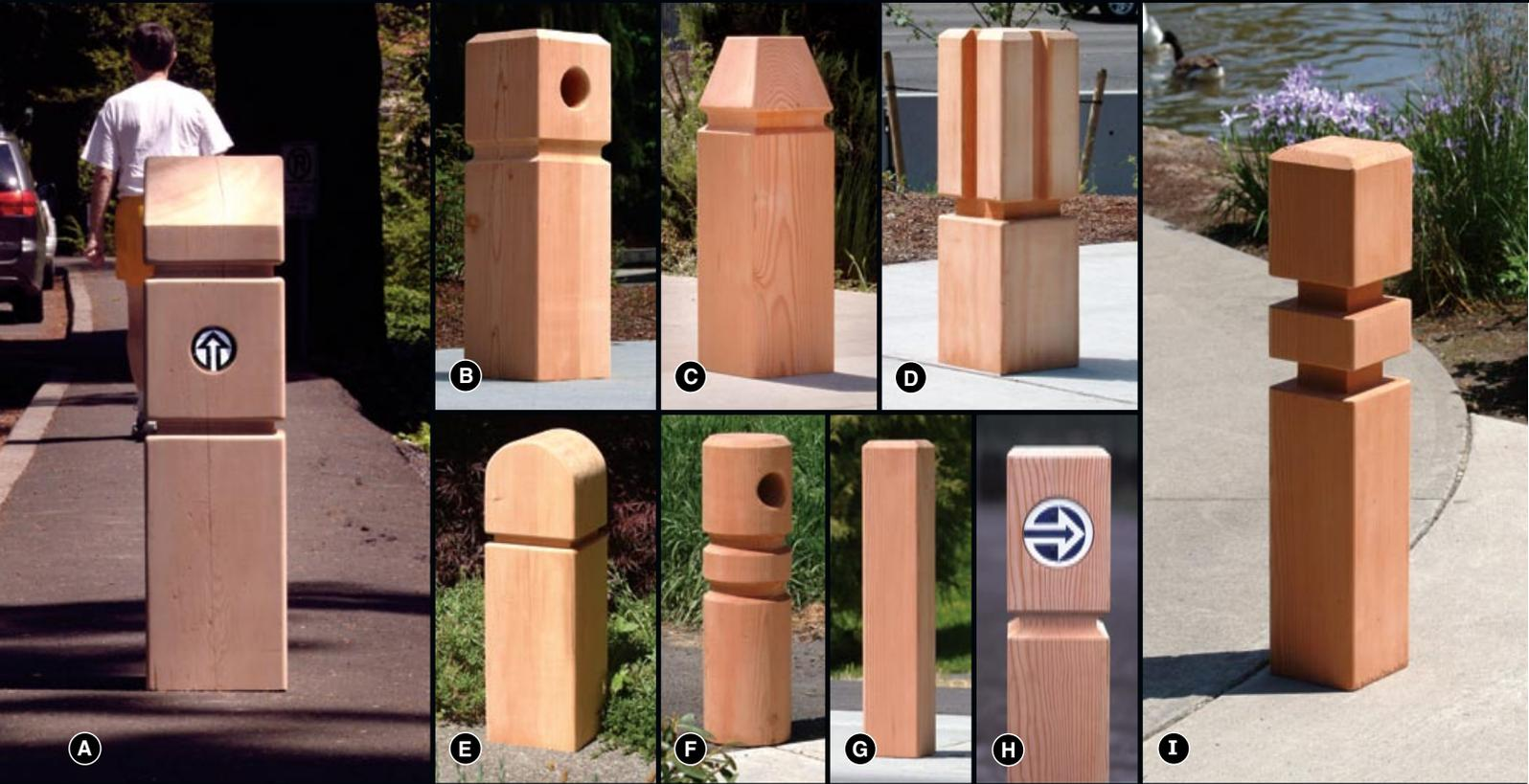
This collection depicts the finest timber bollards available in the world today. Most designs can be made from nominal 8 x 8 (7-1/4" x 7-1/4" net) or 12 x 12 (11-1/4" x 11-1/4" net) free-of-heart-center (F.O.H.C.) Douglas fir timbers. Supplied square or lathe-turned full-length to a constant diameter, these sculpted timbers are offered in (exposed) heights above grade of 2'6", 3'0" and 3'6". Other heights are available.
